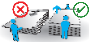
1. Boards need to be handled by 2 people.
